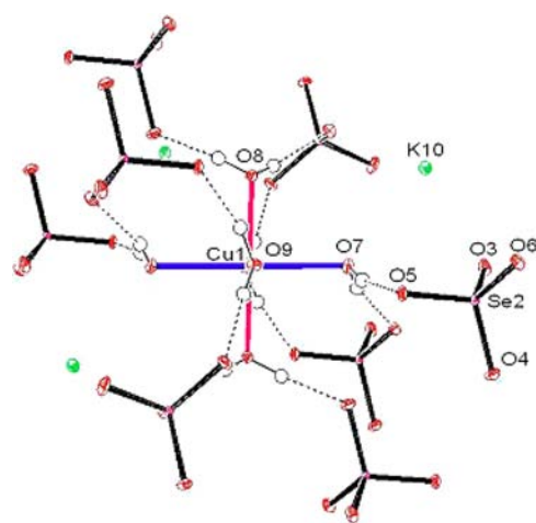
Figure 2. ORTEP drawing of the structure of \text{K}_2[\text{Cu}(\text{H}_2\text{O})_6](\text{SeO}_4)_2 viewed approximately perpendicular to the short Cu–O(9) bond direction. Displacement ellipsoids are drawn at the 20% probability level. There are 12 hydrogen-bonding contacts for each [\text{Cu}(\text{H}_2\text{O})_6]^{2+} complex to eight surrounding selenate counteranions.
